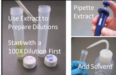
Adjust setting on the micropipette, attach a tip and use a 2nd test tube to prepare a dilution for analysis. Examples shown below account for the dilutions created in Step 1:
