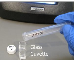
Tighten cap and shake dilution made in Step 3 for several seconds prior to use. Pour dilution into the glass cuvette, about half full. Use a tissue wipe to keep the outside glass clean from liquids or fingerprints. Next, carefully place cuvette into the UV Module and close the lid. Be careful not to spill!
