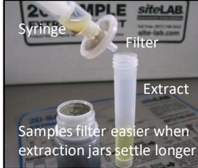
Shake extract jars by hand for several minutes. Next, let jars settle for several more minutes or longer if needed. Remove lid and suck up 2 to 4 mL from the surface using a syringe. Attach/screw a filter to the syringe and dispense contents into a test tube. Label Extract tube with sample ID and 2X or 4X.
