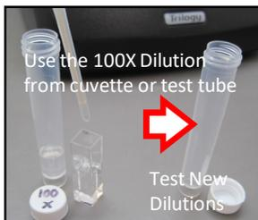
Samples with very high concentrations of hydrocarbons require very big dilutions for analysis. The 100X Dilution prepared in Step 3 can be further diluted using the pipette. Pipette contents of the 100X into a clean test tube and add 5 mL or 10 mL of solvent. Use examples below:
