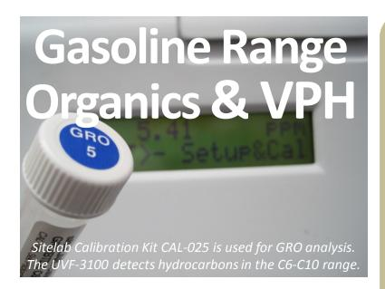
An environmental consulting firm performed a 3-way study testing samples at a former tank farm once used to store gasoline and fuel oils. They wanted to know how Sitelab compares to two different laboratory methods, GRO and VPH, which are commonly used across the US. Sitelab's GRO calibration kit and UVF-3100 optics were developed to correlate well to U.S. EPA and state regulatory test methods for gasoline range/volatile petroleum hydrocarbons.
