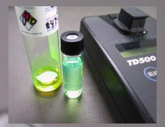
Sitelab's TD-500D analyzer was calibrated to the oil of interest. In some cases, clean parts were detected down below 10 ppb.
