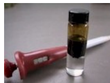
Photo of 40 Oil Sample Extracts at 5,000 ppm in Hexane Solvent Samples contaminated with heavy fuel oil and weathered diesel are dark in color due to high proportions of PAH compounds. Samples with fresher diesel fuel are lighter in color as they contain fewer PAH compounds.
