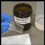
Rinse cuvette with solvent prior to use and place onto tissue wipes. Use a waste cup to collect solvent.
