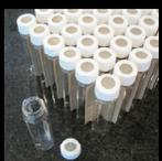
Sample Extraction Vials - Water Product No. EXTR-72-40ML Use for sample analysis. Solvent not included. Use HPLC grade hexane.
