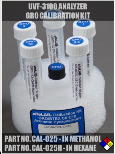
This product contains five linear calibration solutions used for accurate UVF-3100 analysis. A reference standard is also included for backup, used to make new calibration standards if necessary. Sitelab calibration kits are supplied with a <u>3-month</u> or <u>6-month</u> expiration date. GRO minimum detection limit = 0.5 ppm.
