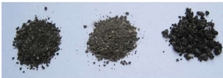
Photo showing asphalt samples provided by a laboratory in France, which they ground and sieved to 2 mm in size for analysis. ADEPT specifies samples be a minimum of 4 mm in size. This small particle size helps ensure samples are well homogenized and improves data quality.
