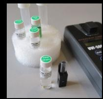
Use to calibrate analyzer for Total Petroleum Hydrocarbons. Detects TPH in the C15 to C50 carbon range. Kit includes:
