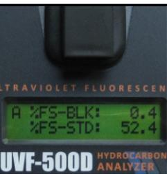
Compare the %FS values to the factory calibration data. %FS values should be close/similar each time the analyzer is calibrated to TPH.
