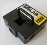
PAHS Module for Target PAHs, EDRO Module for EPH Aromatics
