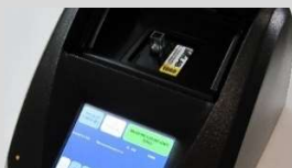
Sitelab UVF-Trilogy Analyzer with EDRO Module Inserted
